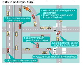
**Example of Driver Support Using Precise Positioning**
