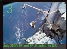
On the third assembly mission, 2J/A (STS-127), the EF and an EP were attached to the ISS. The photograph shows the Monitor of All-sky X-ray Image (MAXI) unit—to be attached to the EF—being manipulated by JAXA Astronaut Koichi Wakata who is operating the JEMRMS robotic arm. The empty EP was returned to ground aboard the Endeavour.
