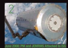
On Mission 1J (STS-124), the second assembly mission for JEM Kibo, the PM was berthed to the ISS and JEMRMS was attached. This photograph shows the PM being gripped by the Space Station Remote Manipulator System (SSRMS)—the ISS' main robotic arm, also known as Canadarm2.
