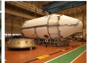
Above: F3 fairing Left: 1 st stage core vehicle
