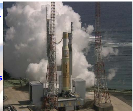
1st stage flight tank stage firing test 18
