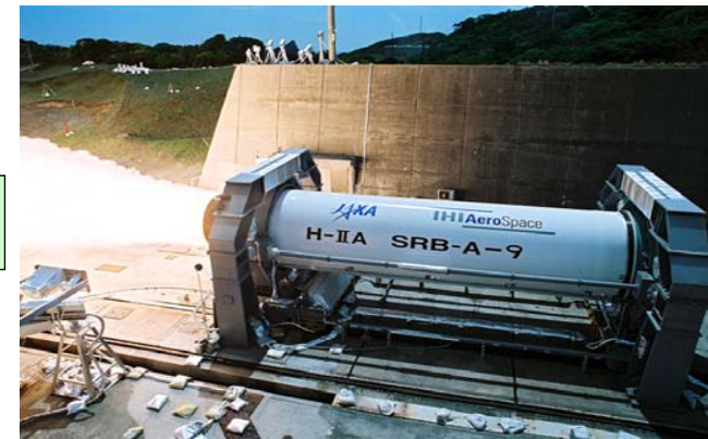
Static firing test of the improved SRB-A
