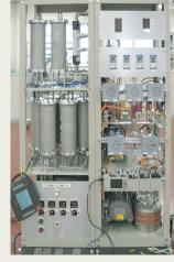
Experimental component to separate and recover CO<sub>2</sub> emitted by one astronaut (right) and a schematic diagram of the system (left)
