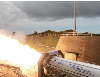
T Takesaki Static Firing Test Facility for Solid Motor This facility is used for conducting ground firing tests of solid rocket boosters that generate a strong propulsion force. The firing tests of the solid rocket booster (SRB-3) of the H3 launch vehicle being developed were conducted here.
