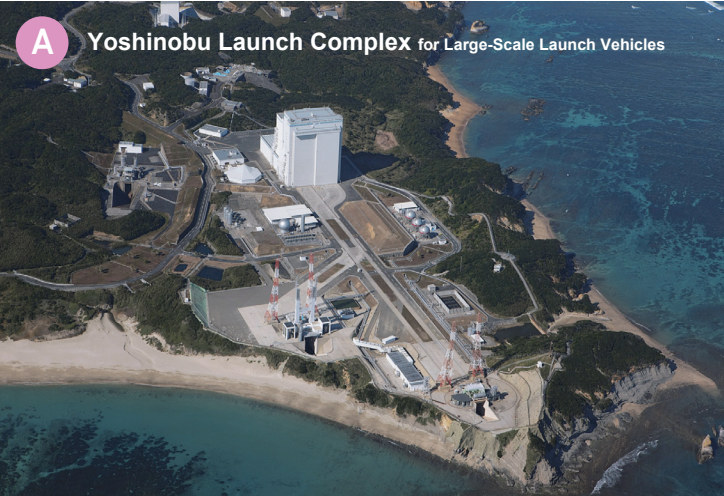
Launch vehicles are assembled, fitted, filled with fuel and launched at the Yoshinobu Launch Complex on the north side of the Tanegashima Space Center.
