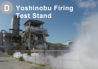
This is the ground firing test site for the first-stage engine, which can be said to be the heart of the rocket. At present, it is used for testing the first stage engine (LE-9) of the H3 launch vehicle being developed.
