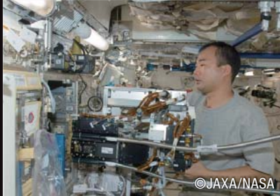
In the Fluid Physics Experiment Facility (FPEF), performing repairs on apparatus used in the "Space-time Structure in Marangoni Convection" experiment
