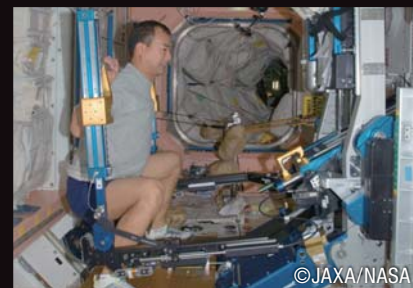
Using the Advanced Resistive Exercise Device (ARED) during a physical workout
