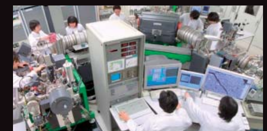
The world's first isotope microscope system was used to analyze the sample from Itokawa.
