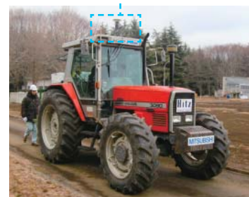
The experiment was held in February 2011 at the National Institute for Rural Engineering, in Tsukuba, with antennae for GPS and MICHIBIKI fitted to the top of the tractor's cab.
