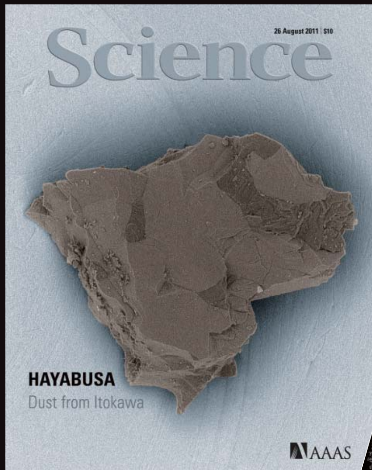
© Science The cover of the August 26, 2011, issue of Science features a photograph of a particle from Itokawa. This image was captured using an electron microscope. This particle of dust, measuring just 181 \times 86 \mu\text{m} , was found to contain such substances as olivine, plagioclase, and iron sulfide.
