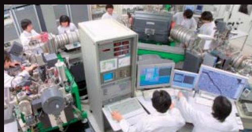
The world's first isotope microscope system was used to analyze the sample from Itokawa.
