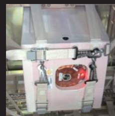
i-Ball loaded onto an HTV Resupply Rack (HRR) in the Pressurized Logistics Carrier (PLC)
