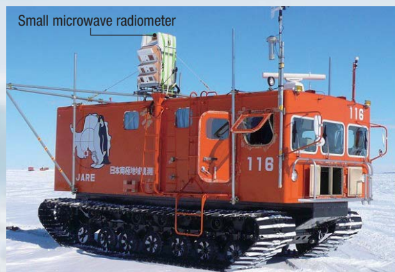
Small microwave radiometers are being used for mobile and fixed-location observations as well as observation experiments
