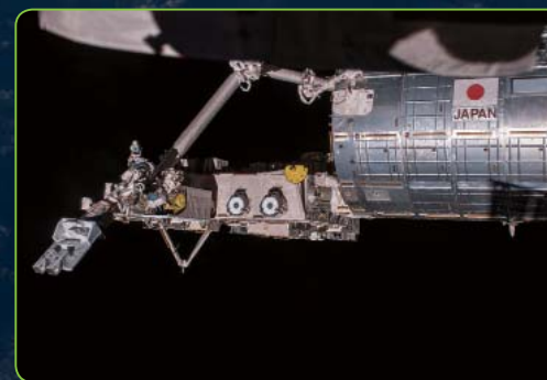
JEM Remote Manipulator System (JEMRMS) grips the JEM-Small Satellite Orbital Deployer (J-SSOD) (© JAXA/NASA)
