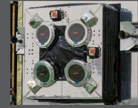
Hayabusa2's ion engines have increased propulsion power compared with Hayabusa, and were designed to have an extended life. (© JAXA)
