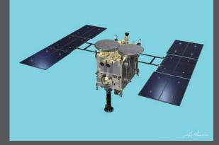
Two large discs that feature on the upper-exterior of Hayabusa2 are an X-band high-gain antenna (left) and a Ka-band high-gain antenna (right) (computer graphic image)
