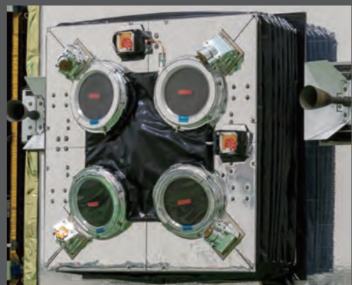
Hayabusa2's ion engines have increased propulsion power compared with Hayabusa, and were designed to have an extended life. (© JAXA)
