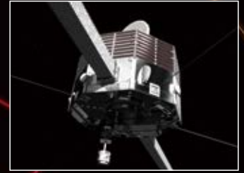
Mercury Magnetospheric Orbiter (MMO) developed by JAXA. The rod-shaped component visible is the magnetometer mast. (© JAXA)
