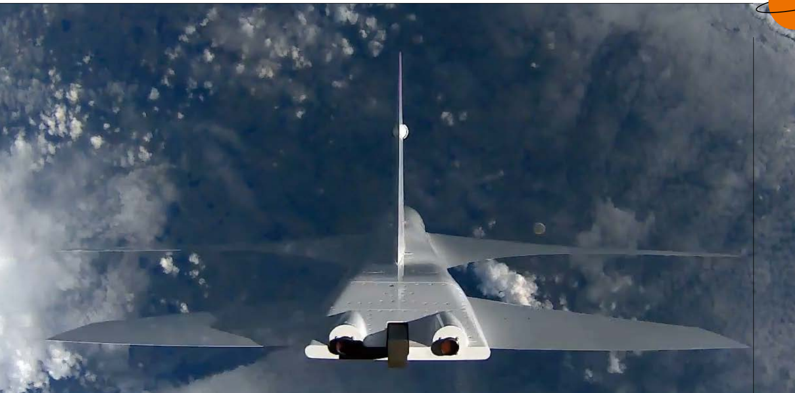
The moment at which the D-SEND#2 experimental aircraft—named the Silent SuperSonic Concept Model (S3CM)—was released from a balloon at an altitude of 30.5 km (© JAXA)
