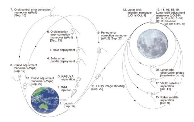
\* Lunar orbit adjustment maneuver (LOI5 and 6): orbit control to lower the KAGUYA's altitude in the injected lunar orbit (18 and 19 in the above figure)
