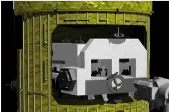
First, the station's robotic arm (SSRMS) will pull out the Exposed Pallet (EP) from the HTV Unpressurized Logistics Module (ULC).
