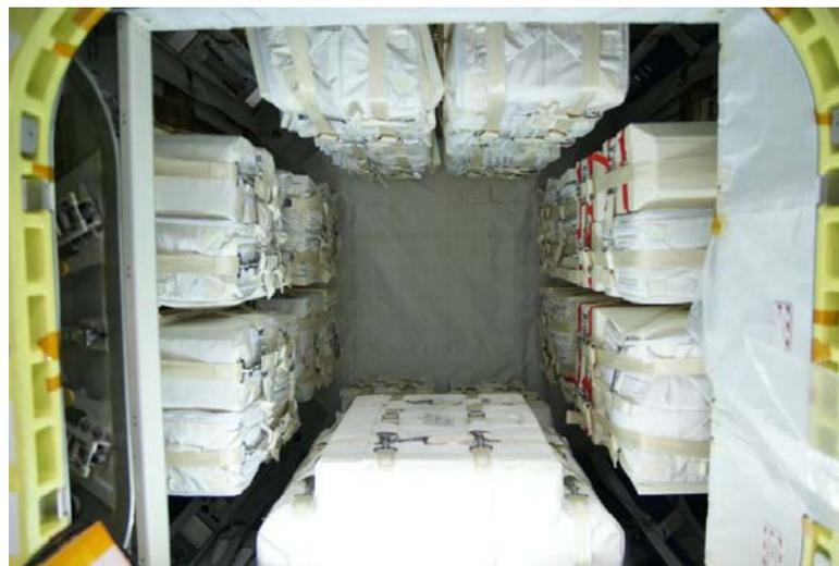
Fig. 2.3.1-6 Cargo Layout inside the PLC (HTV-1)
