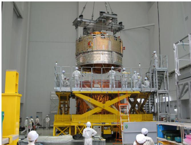
Fig. 1.3.1-3 PLC and ULC being mated
