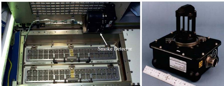
Smoke Detectors will be installed on the ventilation system in the PLC during docked operations
