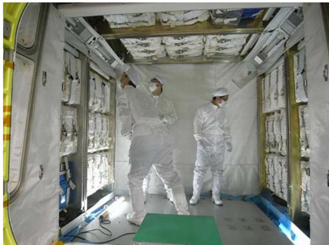
Inside of the HTV Pressurized Logistics Carrier (PLC)
