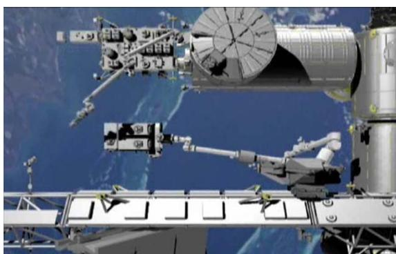
First, Kibo's robotic arm (JEMRMS) will remove the EP from the EF.
