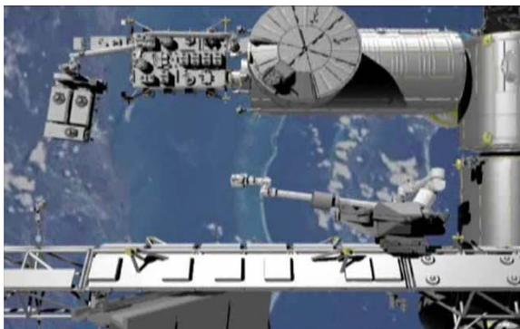
After the payloads are unloaded and relocated to Kibo's EF, the EP will be re-stowed in the ULC.
