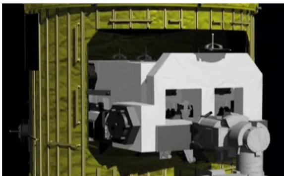
Finally, the EP will be reinstalled in the ULC by the SSRMS.
