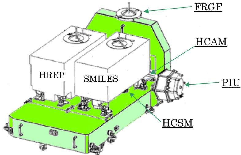
Fig. 1.2.3-3 Exposed Pallet for EF Payload
