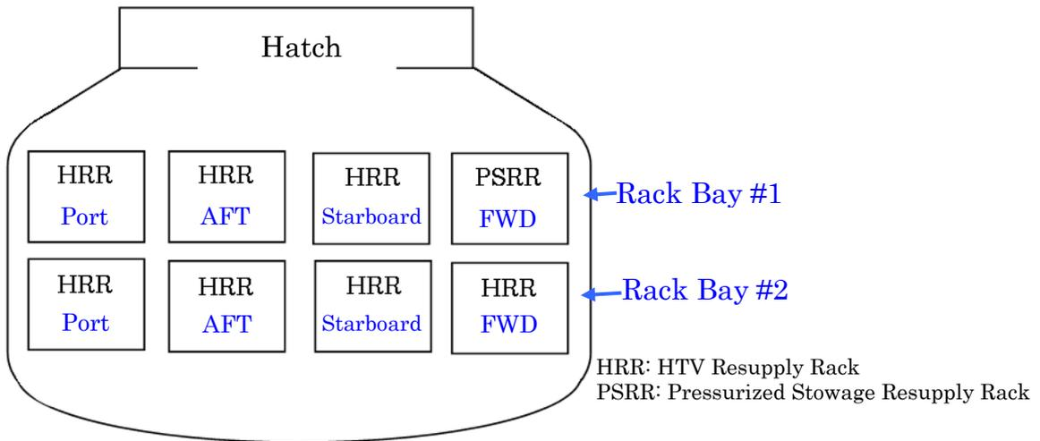
Fig. 1.2.1-3 Rack Layout inside the HTV (HTV-1)
