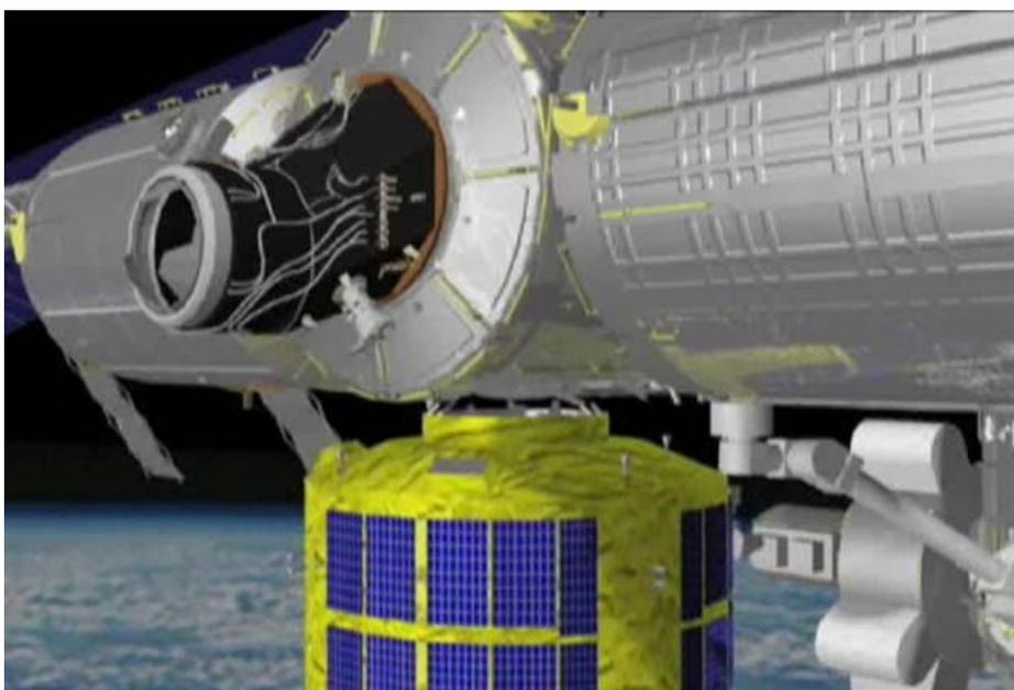
Fig. 1.3.4-5 HTV being berthed to the ISS
