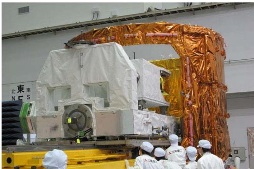
Fig. 1.3.1-2 Exposed Pallet being installed in the ULC
