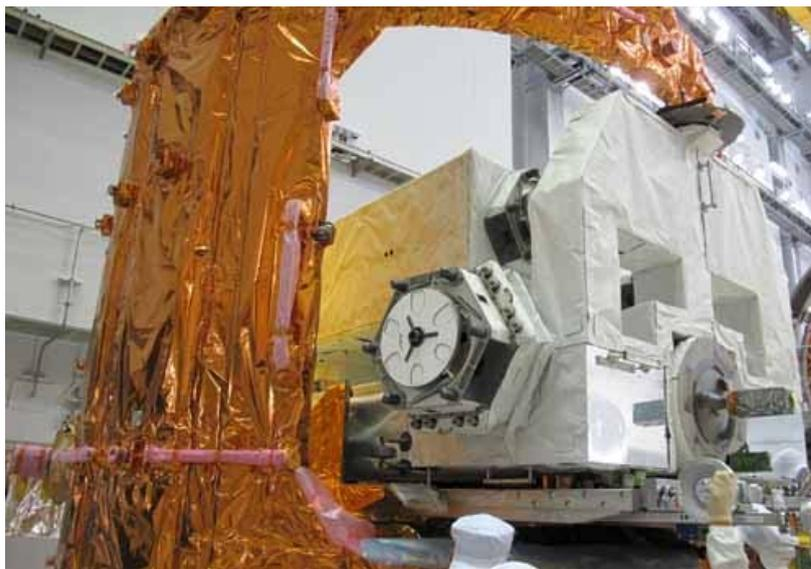
Fig. 1.3.5-2 Exposed Pallet being installed in the ULC
