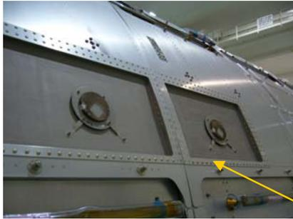
The PROX antennas are used for HTV's direct wireless communications with the ISS during Proximity Operations. It receives telemetry data from the HTV. It is also used to relay the commands sent from the ground or ISS to the HTV.
