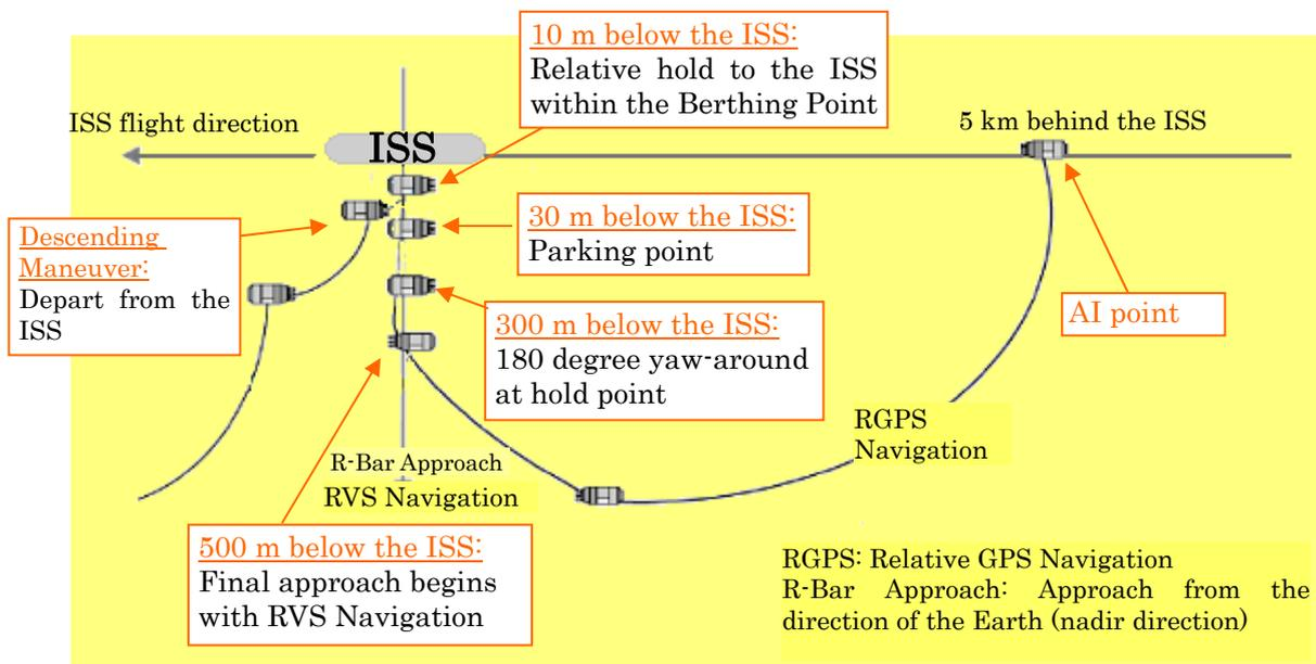
Fig. 1.3.4-1 HTV's RGPS Navigation and R-Bar Approach
