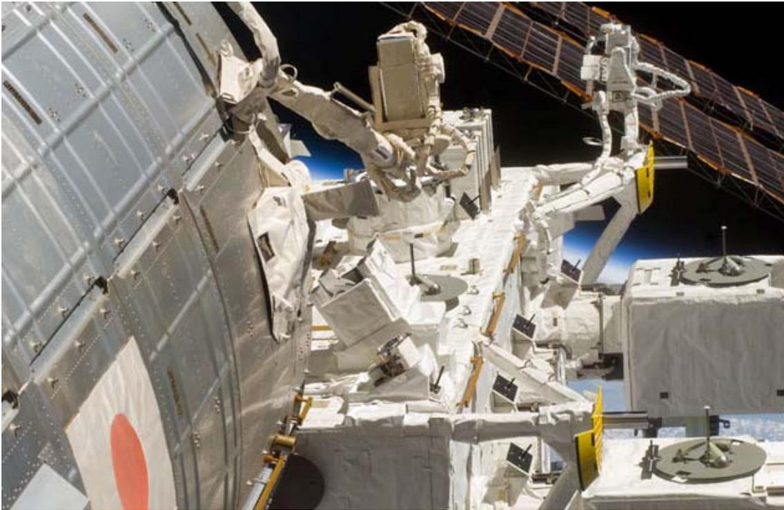
Fig. 2.3.2-5 Exposed Facility (EF) with External Experiments (STS-127)
