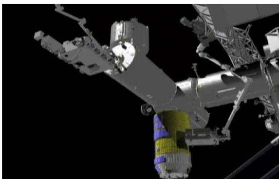
Then, the EP will be handed over to the station's robotic arm (SSRMS).
