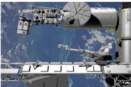
While the EP is attached to the EF, payloads carried on the EP will be relocated to the EF by the JEMRMS.
