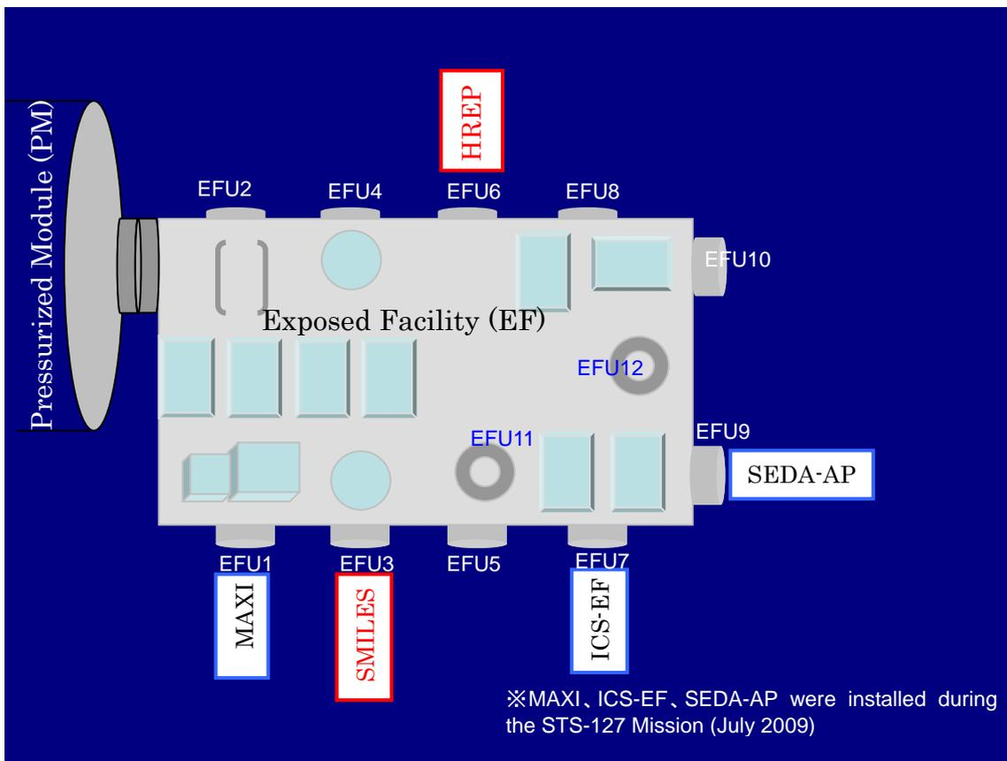
Fig. 2.3.2-4 Attachment Positions of the EF Payloads
