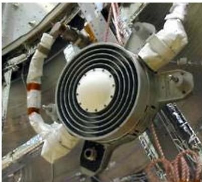
GPS antennas are used to provide information on orbital location and range rate of the ISS to the HTV.
