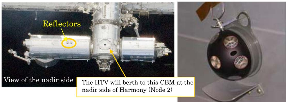
The Laser Rader Reflectors (LRRs) are located on the nadir side of Kibo’s Pressurized Module (PM). The reflectors will reflect the lasers beamed from the HTV’s Rendezvous Sensor (RVS) when the HTV approaches from the nadir side (R-bar) of the ISS.
