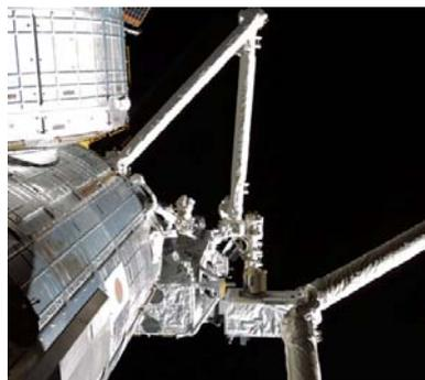
Kibo's robotic arm, JEMRMS, installing an external payload
