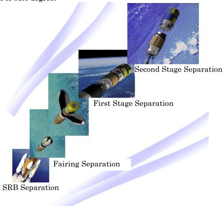
Approximately 15 minutes and 11 seconds after launch, the Second Stage will separate from the HTV. The HTV will then automatically activate the HTV subsystems, maintain its attitude, and perform a self-check on HTV components. After that, the HTV will establish communications with the NASA's TDRS and initiate communications with the HTV Mission Control Room (MCR) at Tsukuba Space Center (TKSC).
