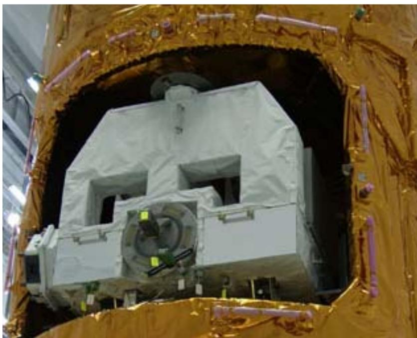
Fig. 1.2.3-2 EP Installed in the ULC
