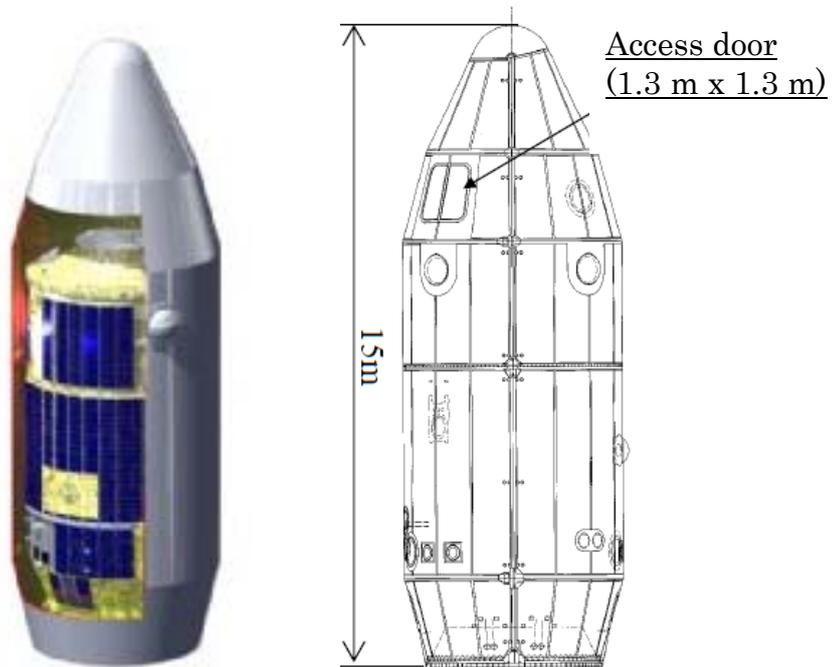
Fig. 1.3.1-5 HTV Installed in H-IIB Rocket Fairing (Image: left)
