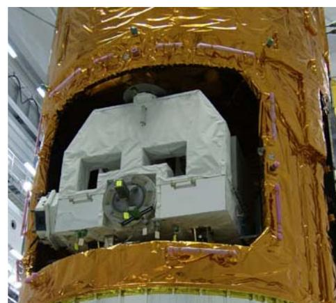
Figure 1.2.2-3 EP Installed into the ULC (HTV-1)
