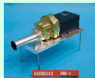
Optical navigation camera, ONC-T
