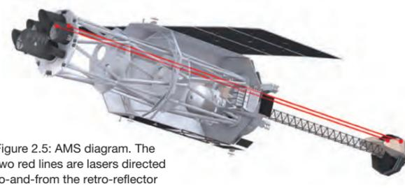
Figure 2.5: AMS diagram. The two red lines are lasers directed to-and-from the retro-reflector
