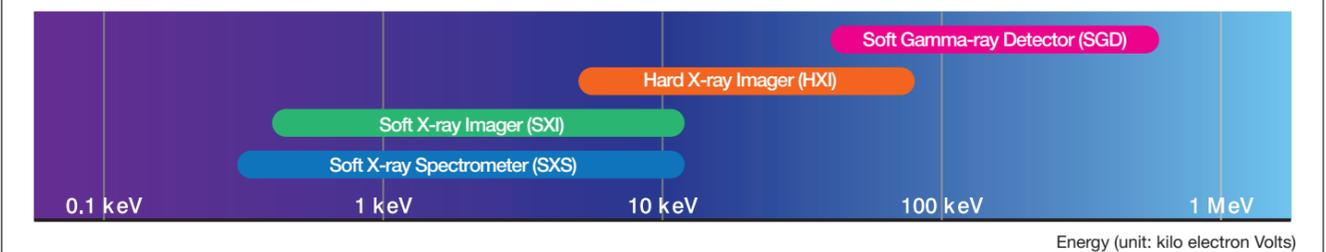
Figure 2.2: Energy range of the 4 detectors on ASTRO-H
