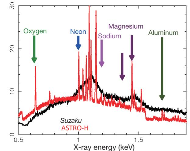
Figure 1.11: X-ray spectra from the Perseus cluster. Suzaku data is from a real observation. ASTRO-H data is a simulation and allows us to detect emission lines from rare elements, such as sodium, aluminum, and to determine abundances accurately.
