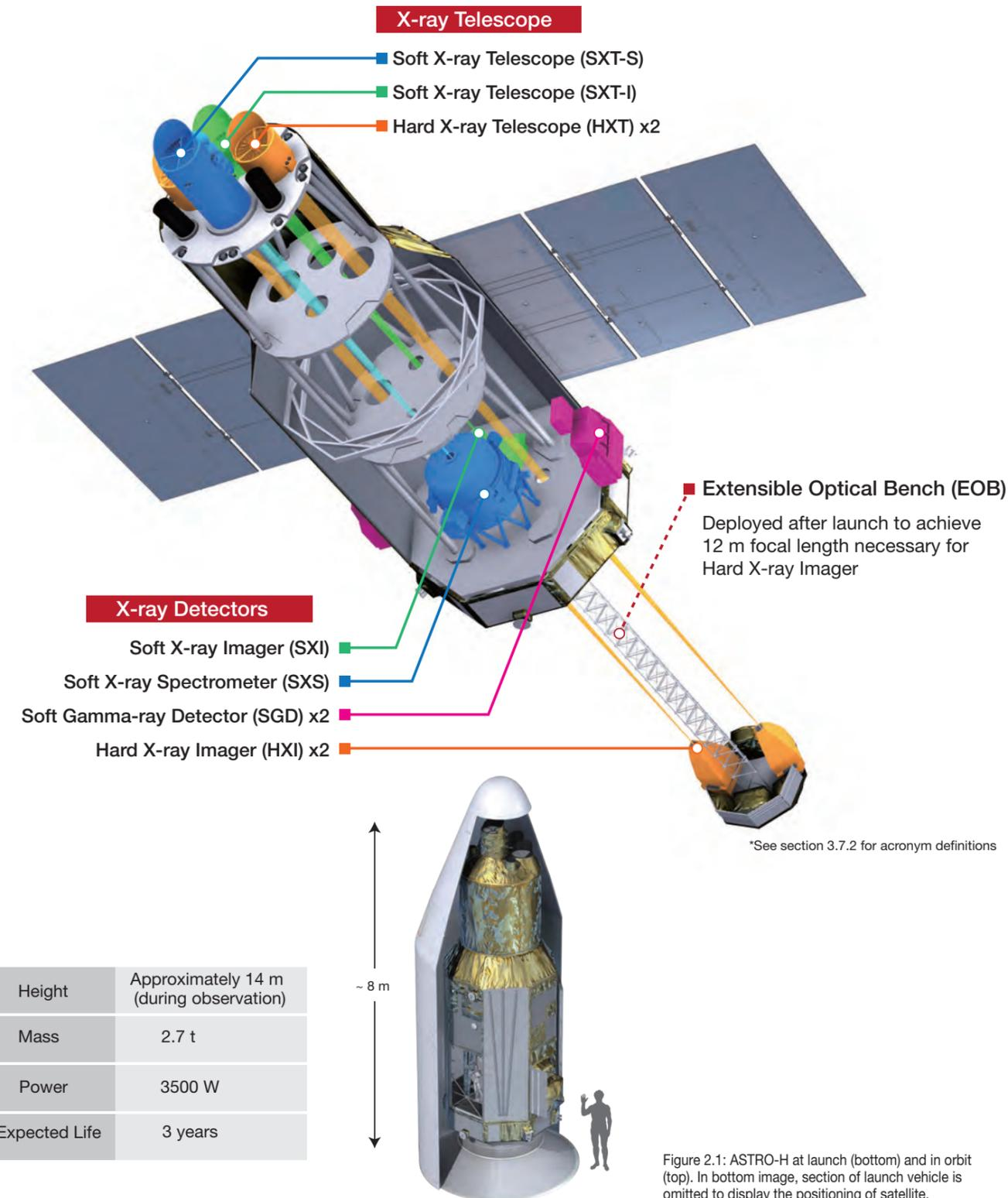
Figure 2.1: ASTRO-H at launch (bottom) and in orbit (top). In bottom image, section of launch vehicle is omitted to display the positioning of satellite.
