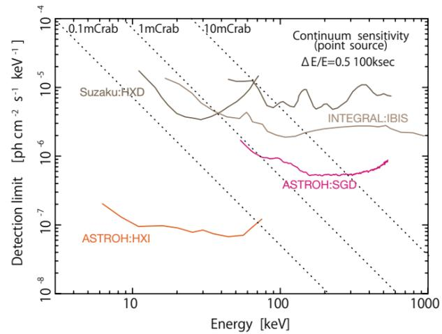
Figure 3.4: Energy band and limiting sensitivity of ASTRO-H hard X-ray/soft Gamma-ray instruments. Suzaku and INTEGRAL (ESA) are also shown for comparison. HXI and SGD have 100 and 10 times greater sensitivity over Suzaku, respectively.
