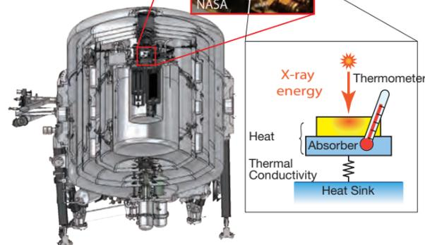
Figure 2.8: Cross-sectional diagram of SXS cooling system
