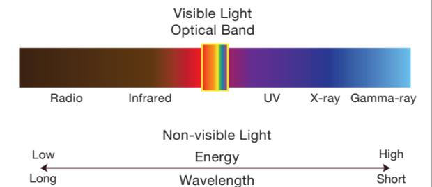
Figure 1.4: Electromagnetic spectrum in energy and wavelength
