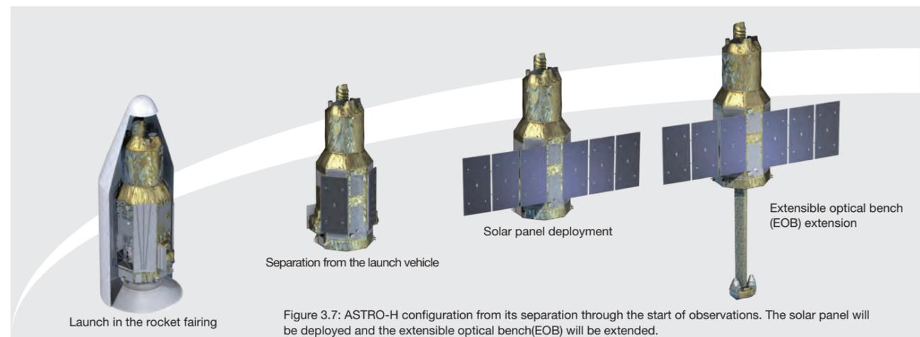
Figure 3.7: ASTRO-H configuration from its separation through the start of observations. The solar panel will be deployed and the extensible optical bench (EOB) will be extended.
